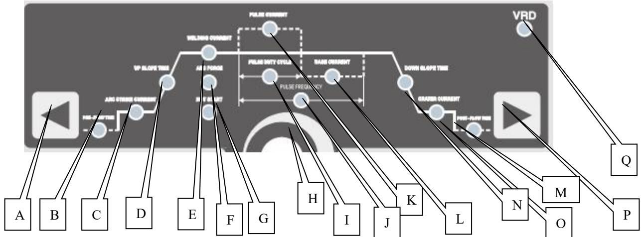
At one time, there is only one indicator light on in this area, which indicates current displayed & adjusted parameter, and the parameter value is displayed on 1st digital display meter, adjusted by encoder. display the welding current in default; When work as MMA or TIG without pulse, it displays the welding current, when work with pulse, it displays the peak current in default.
