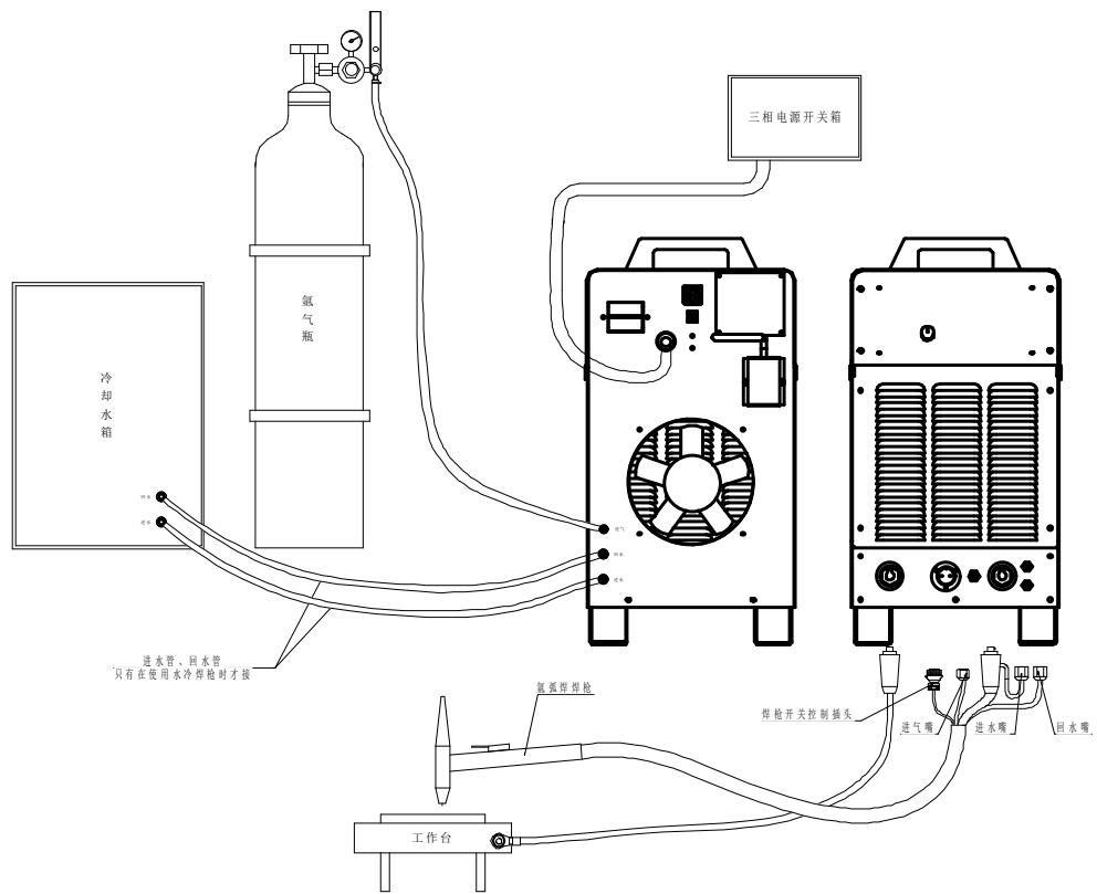
6.2 The power supply of this machine is 3~380V 50/60HZ, user should prepare the switchboard and install the air switch (breaker) and ground cable. Connect the green-yellow wire of the three-phase input cable to the grounding wire on the switchboard reliably according to the below table:
