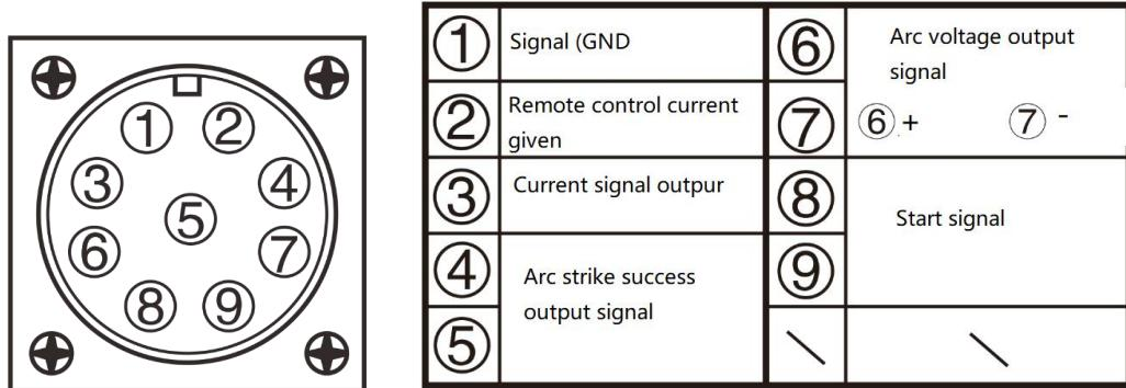
View of the analog communication interface of the welder backplane
